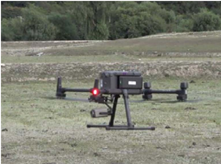
From Sep 2017, UAS flight inspection trial flights for navaid lighting in Qinghai, Tibet and Beijing.
