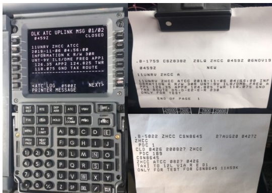
Figure 4 Datalink Air Traffic Control Services in MCDU
