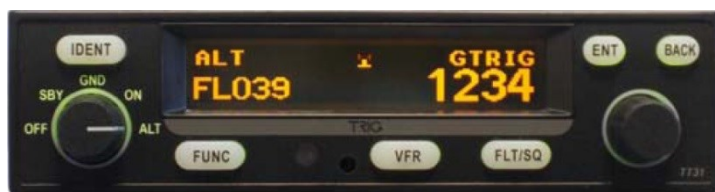
Figure 3.4 TT31 Mode S Transponder from TRIG
