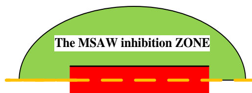
Figure 5: the MSAW Inhibition Zone of the Runway
