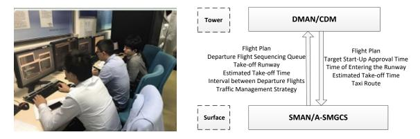
1.10 At present, China is exploring the integrated management of AMAN, DMAN, and SMAN. The basic interaction logic of the three systems is shown in the following figure:
