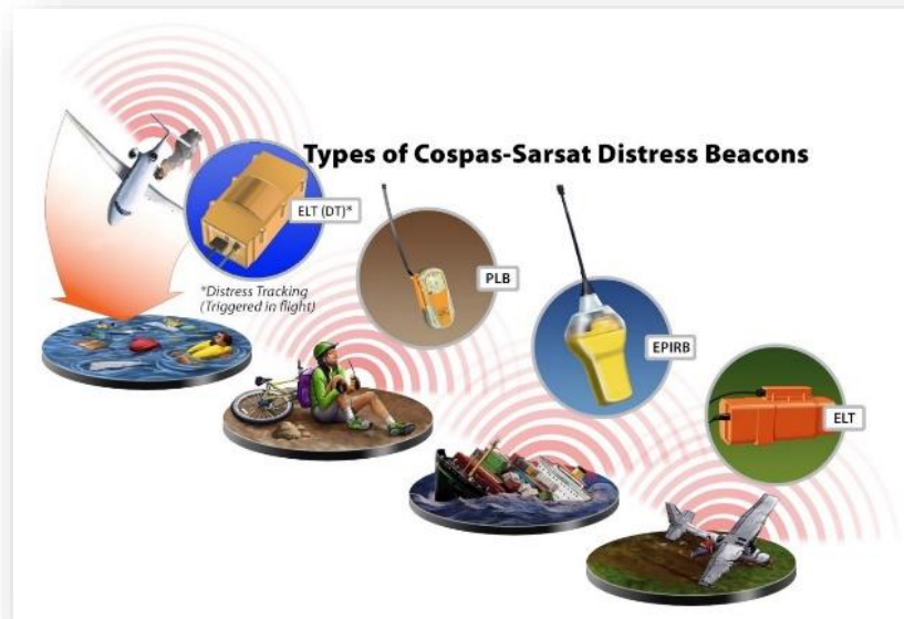
Figure 3: Cospas-Sarsat beacon “types” now include the ELT(DT) for distress tracking
