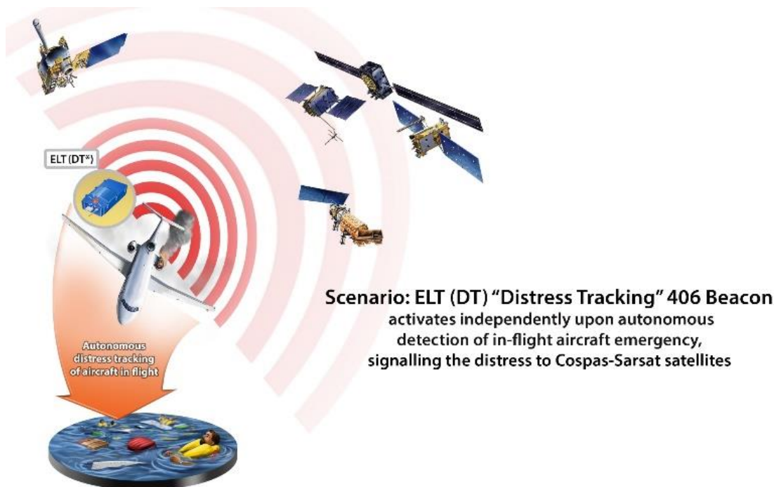
Figure 1: The ELT for Distress Tracking (ELT(DT)) operational scenario
