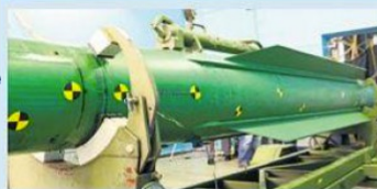
2. Stabilizing fins. (Source: NBAAI)
