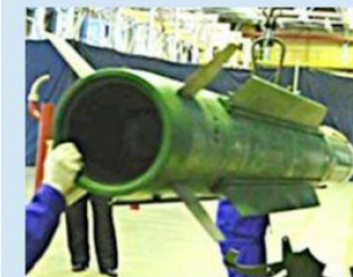
1. Rear nozzle of the missile's engine. (Source: NBAAI)
