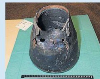
Missile engine nozzle as found in Ukraine. (Source: Dutch Safety Board/Dutch National Police)
