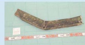
Part of stabilizing fin during identification at Gilze-Rijen Air Force Base. (Source: Dutch Safety Board/Dutch National Police)
