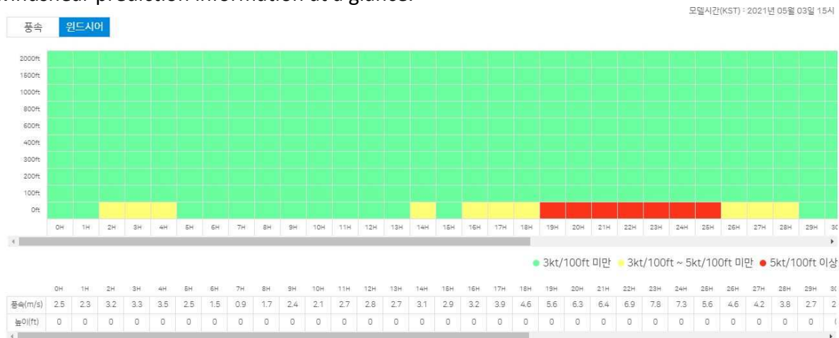
Fig 3. Display screen showing windshear information for Jeju Airport
