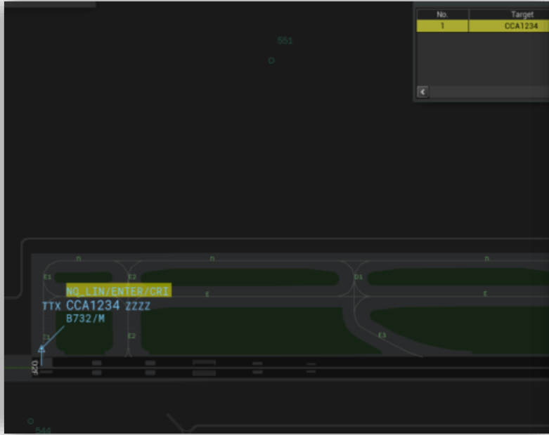
No ENTER clearance warning
