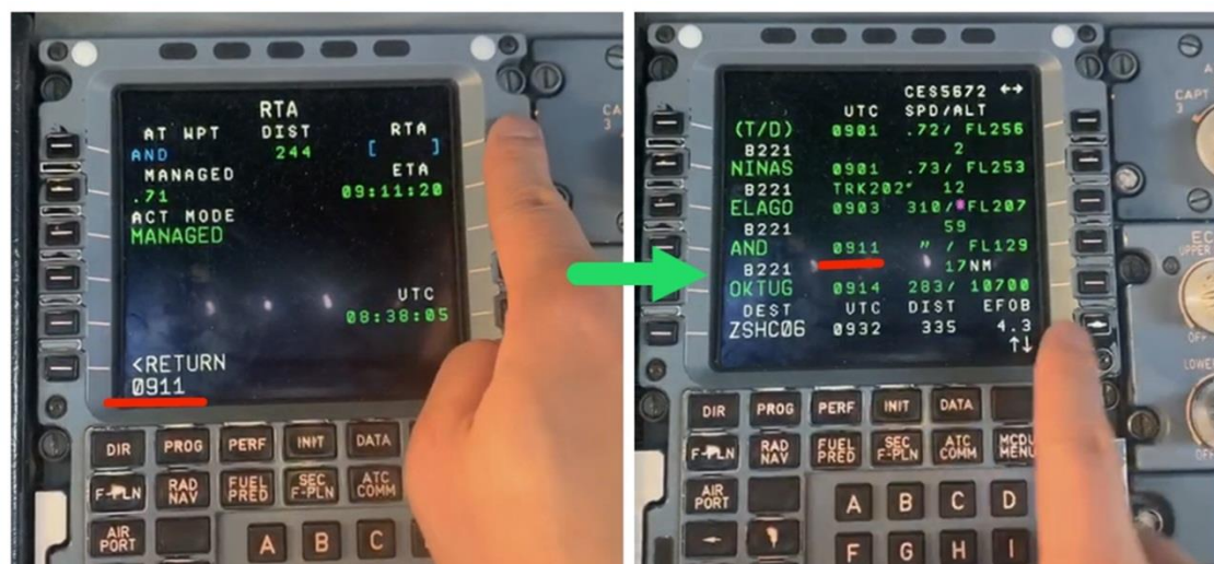
Figure 4: The pilot input the RTA (Required Time Arrival) which issued by ACC controller.
