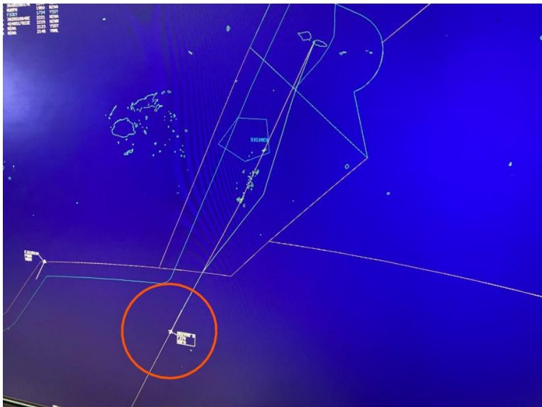
Figure 3. Air New Zealand flight ANZ990 (circled) en-route from Auckland New Zealand to Faleolo International Airport Samoa, was initially on a route that would intersect with SIGMET 10 describing volcanic ash emitted from Tofua. A re-route option was offered by Auckland Oceanic Control, taking the route further east of the SIGMET area.
