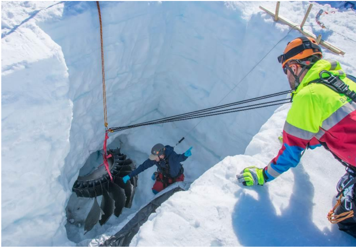
Figure 1: extraction of fan hub fragment (source: Austin Lines)
