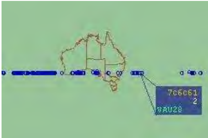
Figure 1 - Track Jumping problem with TPR901
