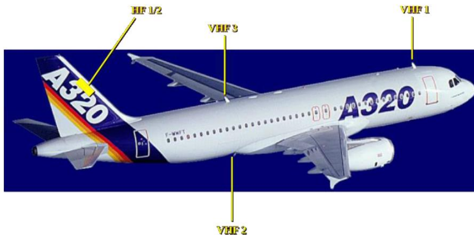
Figure 2 : example of VHF antenna placement on aircraft
