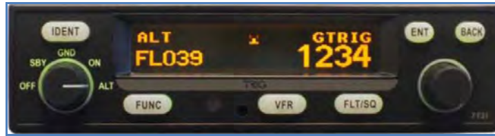
Figure 3.4 TT31 Mode S Transponder from TRIG
