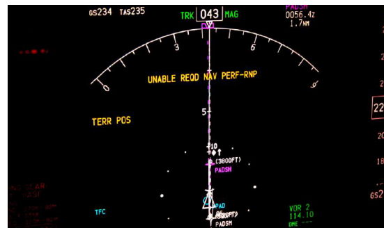
Alert annunciated on Boeing 737NG navigation display
