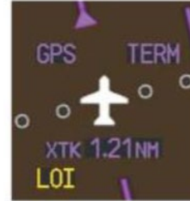
Loss of Integrity Alert for a Garmin G1000 (source: Garmin)
