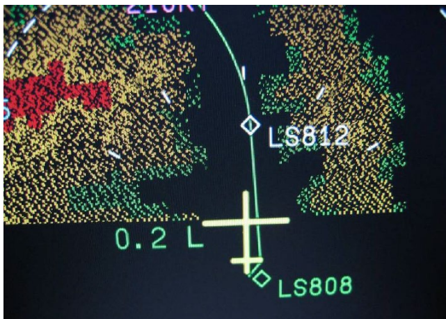
Example of cross-track deviation display in 1/10 th NM
