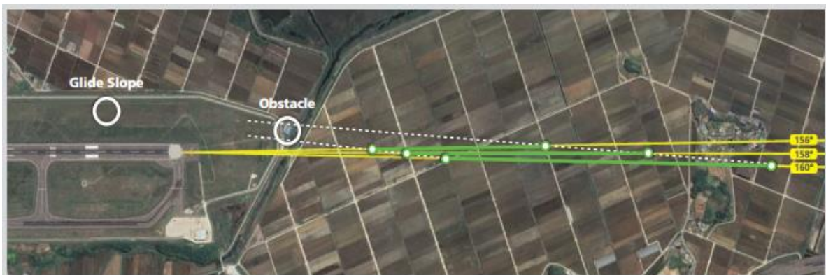
Figure 3. Example of surveying the air wave environment using drone
