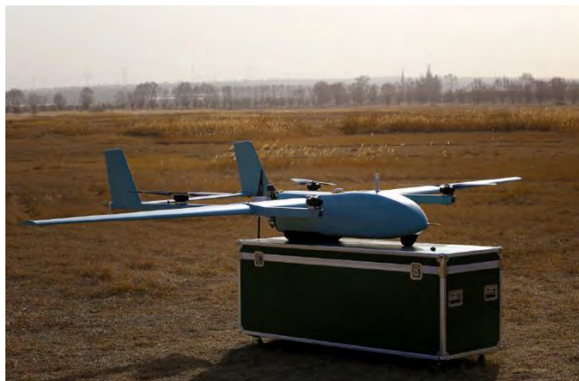
Figure 2 VTOL RPAS used in the project
