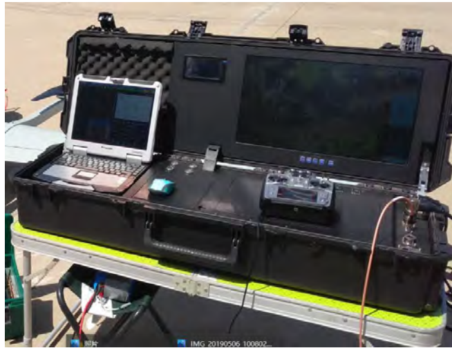
Figure 3 Telecontrol and telemetry station
