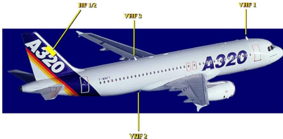
Figure 2 : example of VHF antenna placement on aircraft
