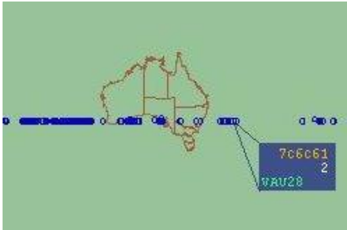
Figure 1 - Track Jumping problem with TPR901
