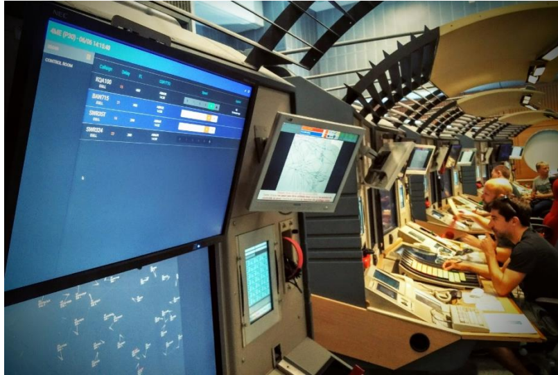
4Me @ DSNA (Reims): on all CWP's in all French ACCs, used for XMAN, tactical ATFM, NM data
