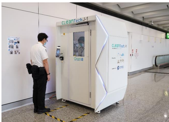
Fig 1. “CLEanTech” disinfection channel
