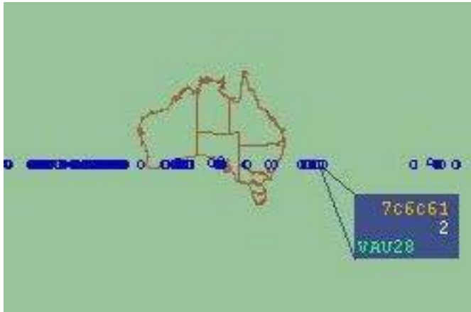
Figure 1 - Track Jumping problem with TPR901
