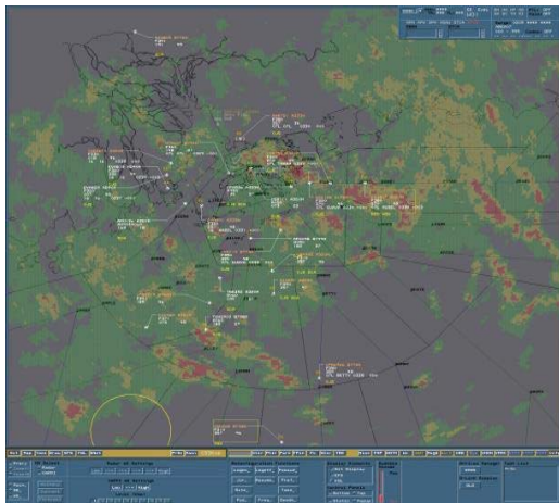
Figure 1. ATC console display showing aircraft positions overlaid on a CAPPI imagery
