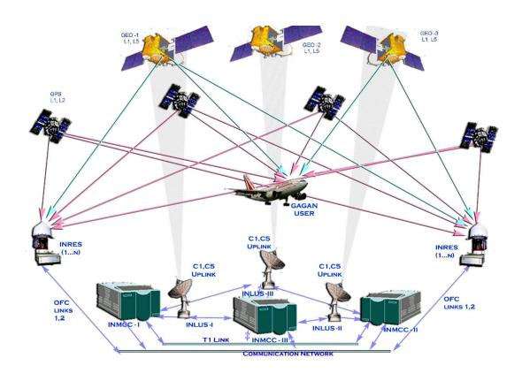
The GPS information collected by these 15 reference stations is forwarded to the INMCC by redundant terrestrial networks. At INMCC, GPS information is processed, and correction (augmentation) messages are generated.
