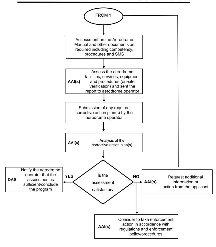
Figure. 1-1: Work Flow Process for the Surveillance of an Aerodrome
