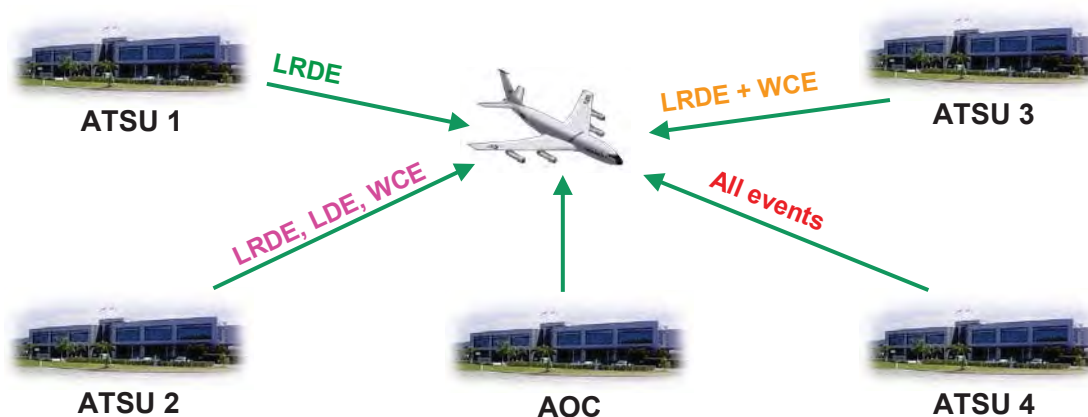
Figure 2-49. Multiple and different ADS event contracts
