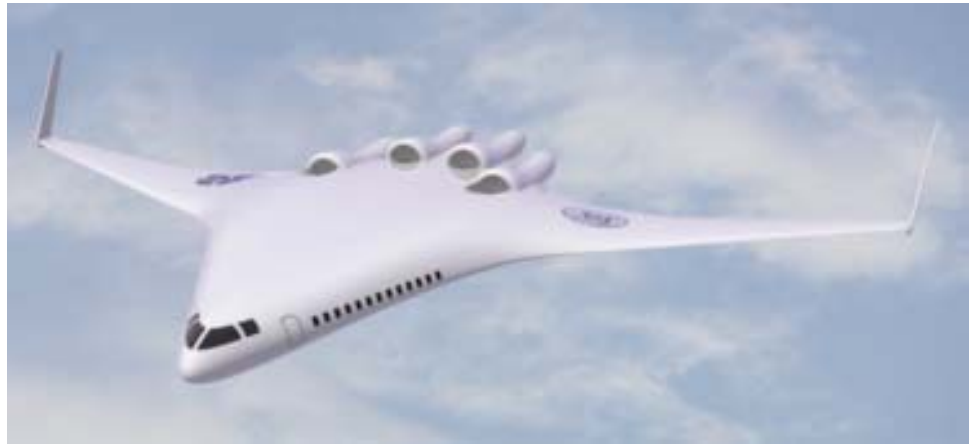
CAD rendering of a “silent” aircraft design features an airframe and engine configuration that is radically different from existing designs. A final conceptual design is expected to be ready for industry review in autumn 2006.
