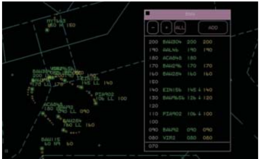
Figure 3. A new tool for managing aircraft holding patterns utilizes downlinked aircraft parameters in the EHS environment.
