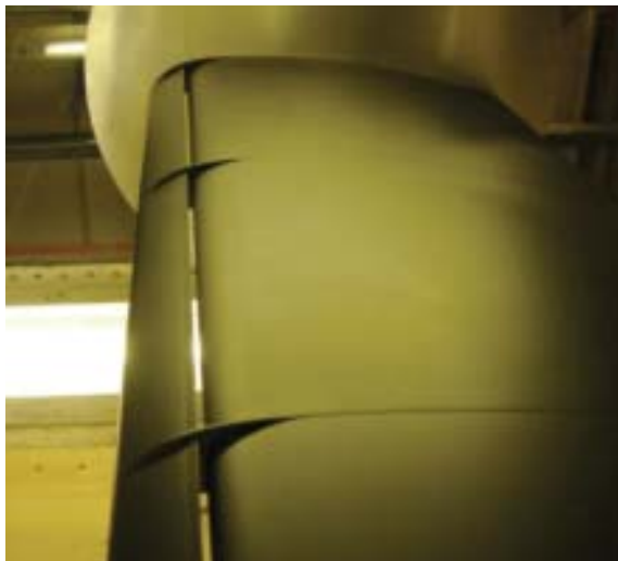
Baseline (conventional) wing slat and high-lift system mounted in a wind tunnel for noise assessment.
