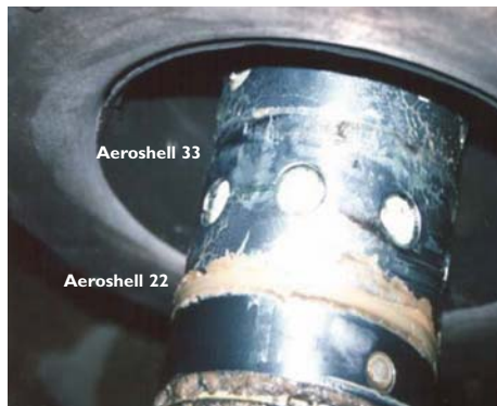
Examination of the wheel axle revealed the presence of two different types of grease, one a general purpose grease (Aeroshell 33) that was not approved for use in this part of the landing gear.
