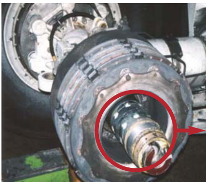
Examination of the wheel axle revealed the presence of two different types of grease, one a general purpose grease (Aeroshell 33) that was not approved for use in this part of the landing gear.
