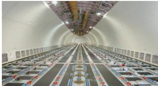
Main Deck Cargo Compartment "Class E"
