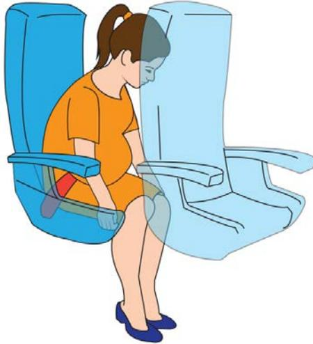
**Figure 16 – Aft-facing seat, lap strap only, high density seating, pregnant passenger**
