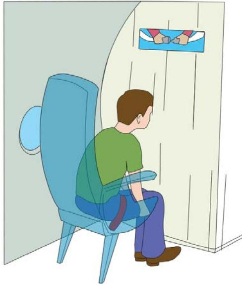
**Figure 6 – Forward-facing seat, lap strap only, high density seating, head against seat back, arms at side**
