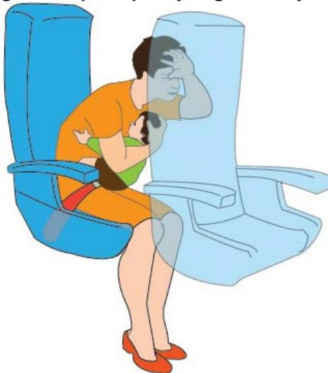
**Figure 28 – Forward-facing seat, lap strap only, high density seating, pregnant passenger**
