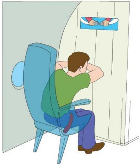
**Figure 26 – Forward-facing seat, lap strap only, high density seating**
