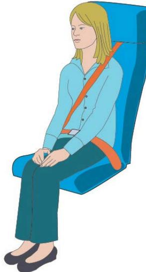
**Figure 19 – Aft-facing crew member seat, lap strap and shoulder harness with dual upper torso straps**
