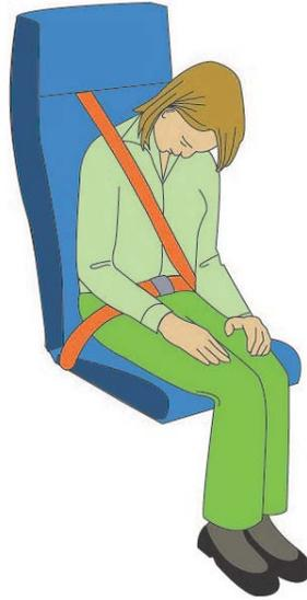
**Figure 8 – Forward-facing crew member seat, lap strap and shoulder harness with dual upper torso straps**
