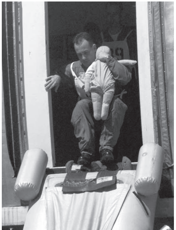
Figure 16. Infant carrier steadies himself as he sits on slide to board; dummy's back is without support or protection.
