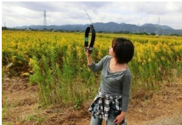
Collar-type transceiver (GPS, 150MHz)
