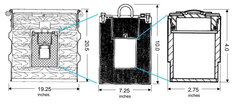
• Steel over-pack with wooden inserts (for impact and thermal protection)
