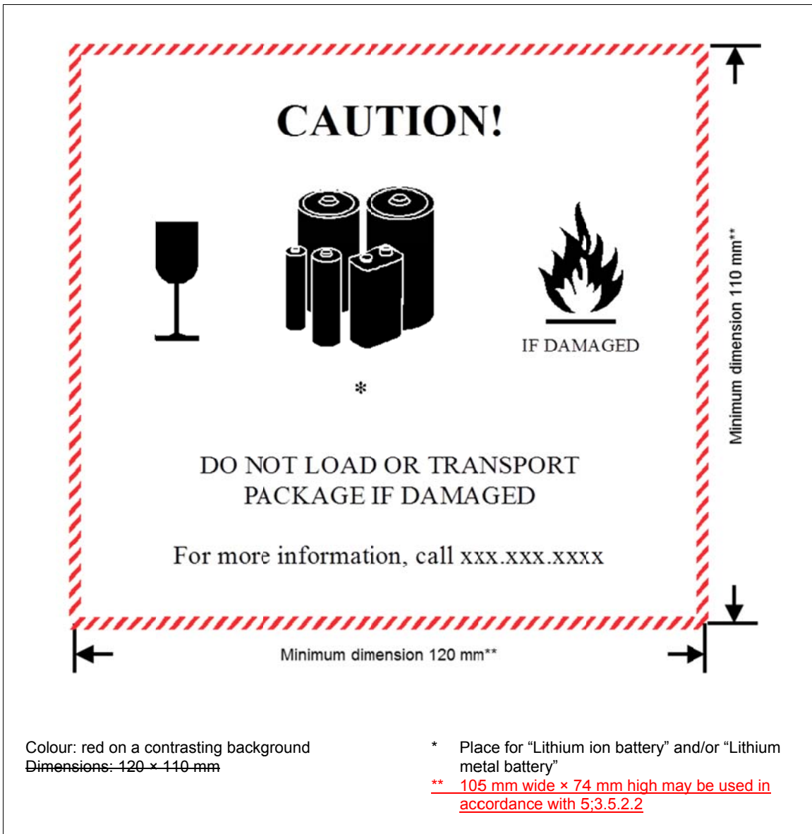
Figure 5-31. Lithium battery handling label
