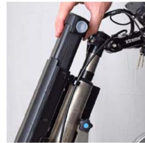
36V Evo batteries Are locked to the frame with a key and have an on-off button on the case
