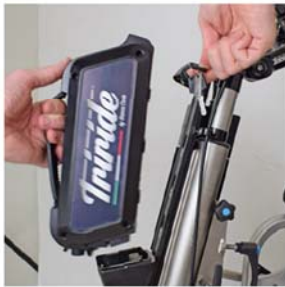
36V and 48V batteries Are locked to the frame with a key and have an on-off button on the case
