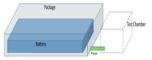
As an alternative to a complete package test, a sub-system may be tested instead. The sub-system shall consist of a set of components which are thermally, mechanically and/or electrically connected such that the subsystem behavior accurately replicates the complete package behavior for the specific test
