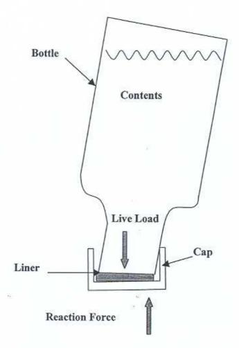
Figure 11: Localized Compression of the Liner
