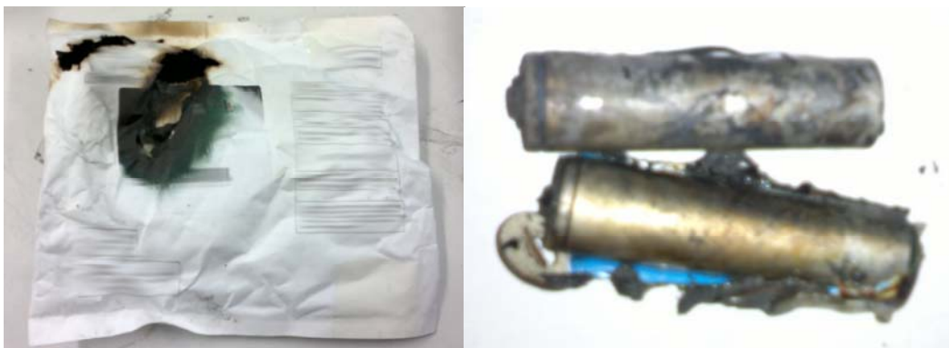
Figure 4 – Fire damage of two undeclared lithium ion cells sent inside an envelope
