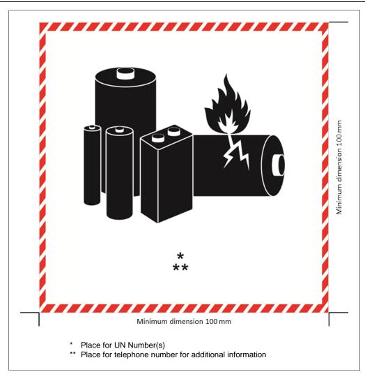
Figure 5-3. Lithium battery mark
