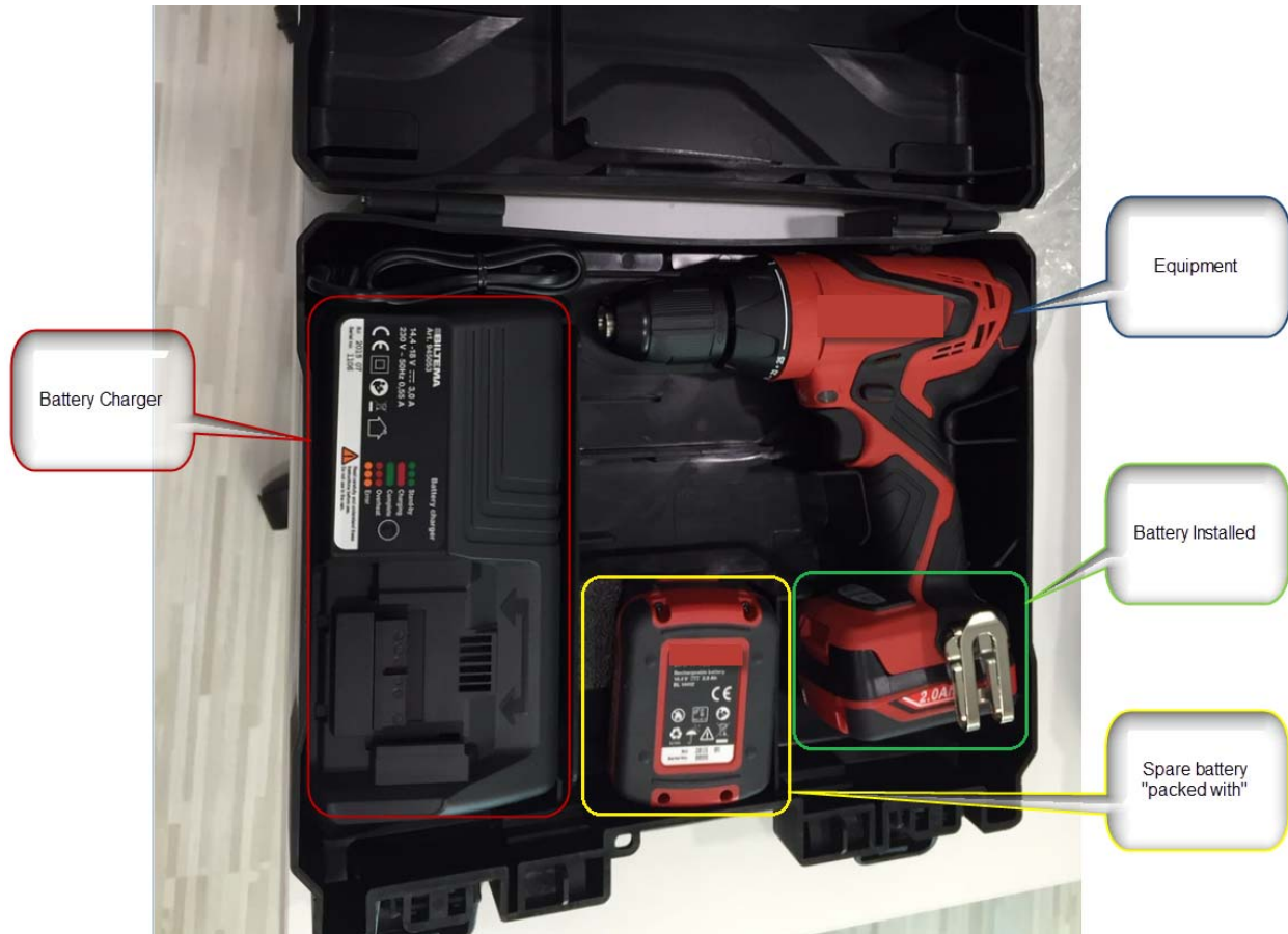
Figure 1 - Example of a power tool with battery installed and one spare battery
