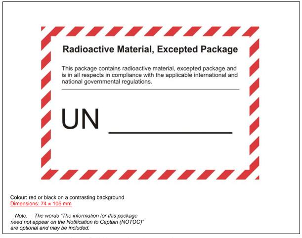
Figure 5-2829. Radioactive material, excepted package
