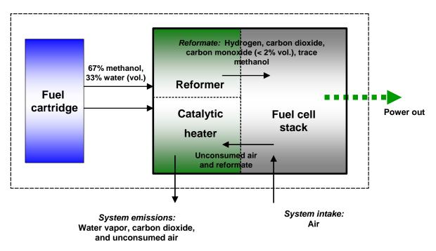
Figure 6. Detail of gas and liquid flows in RMFCs
