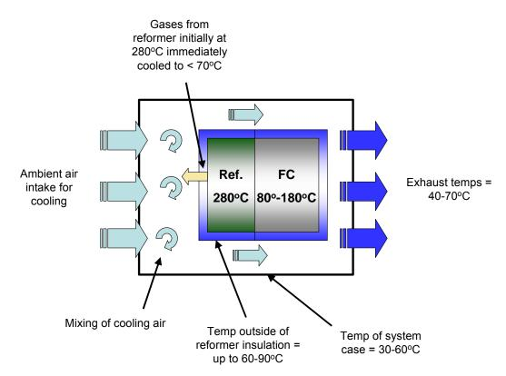
Figure 4. Thermal management in a micro RMFC
