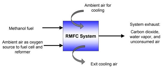
Figure 3. Liquid and gas flows in an RMFC
