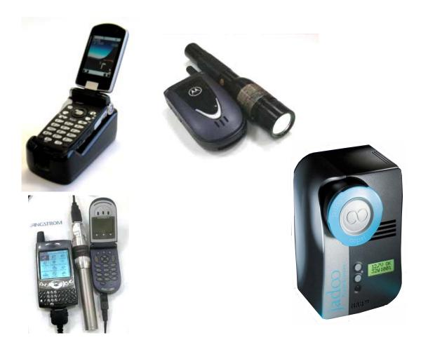
Figure 4: Hydrogen Powered portable electronics devices. Left: Outboard Charging devices, Middle: Fuel Cell Powered flashlight Right: Professional Video Camera Power Supply<sup>3</sup>
