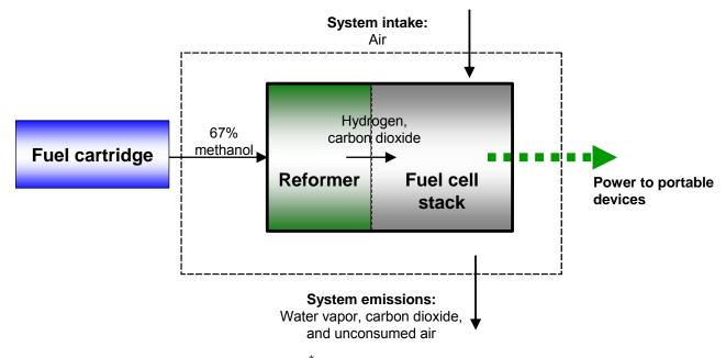
**Figure 1.** Basic schematic of a micro RMFC<sup>\*</sup>
