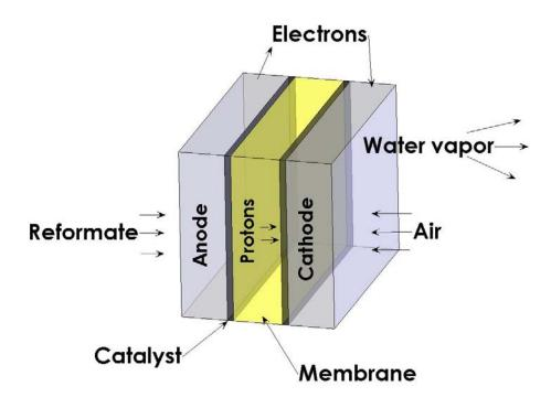
Figure 2. Diagram of a single cell
