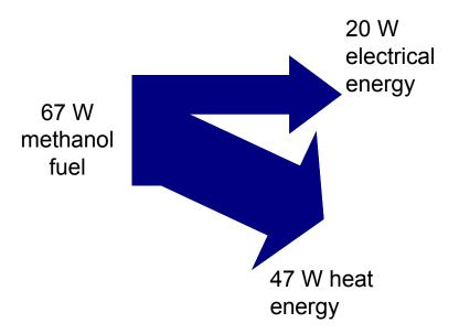
**Figure 5.** Energy flows for a 20 W RMFC and DMFC systems running at equivalent net efficiencies
