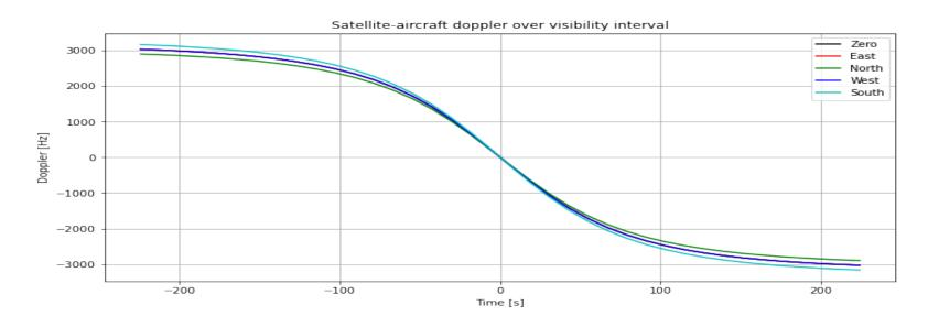
Doppler shift and Doppler rate experienced by an aircraft as function of time in a spacecraft overflight when flying from North to South
