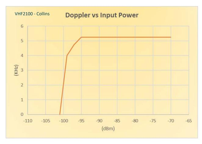
Maximum Doppler shift at the receiver input for which the VDL2 link is established and maintained for different input powers
