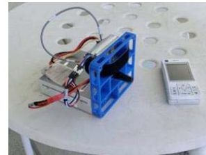
Onboard wireless relay station (OWRS)
