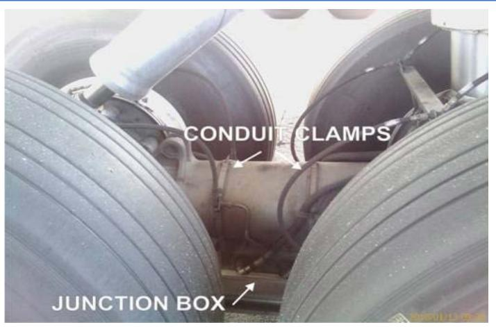
Junction box clamps on 777 truck beam susceptible to water impingement due to ponding.
