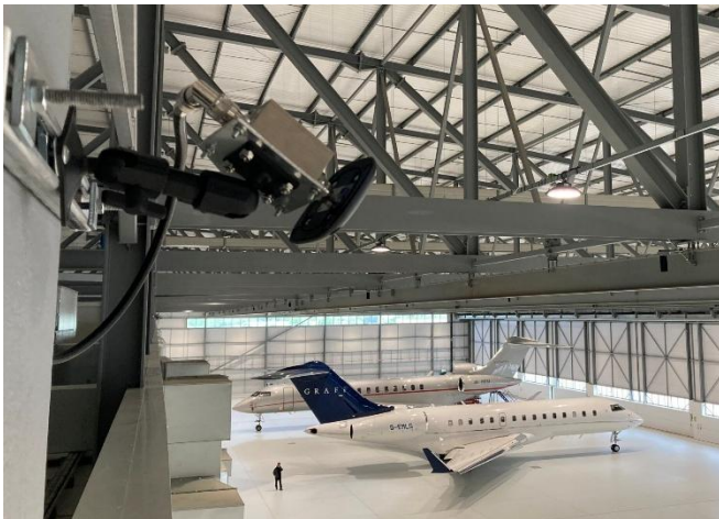
S1 spoofing scenario : GNSS repeater
