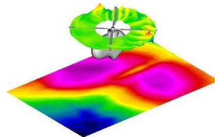
Figure: Load distribution on rotor and noise carpet below wind tunnel model.
