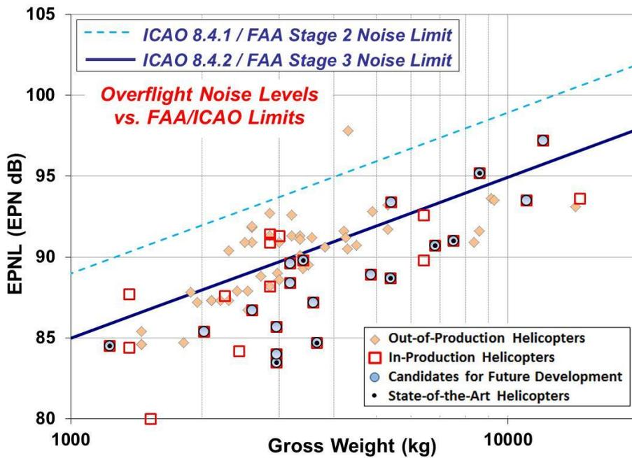
Figure A-3. Chapter 8 Overflight Certification Noise Levels vs. 8.4.1 and 8.4.2 Noise Limits
