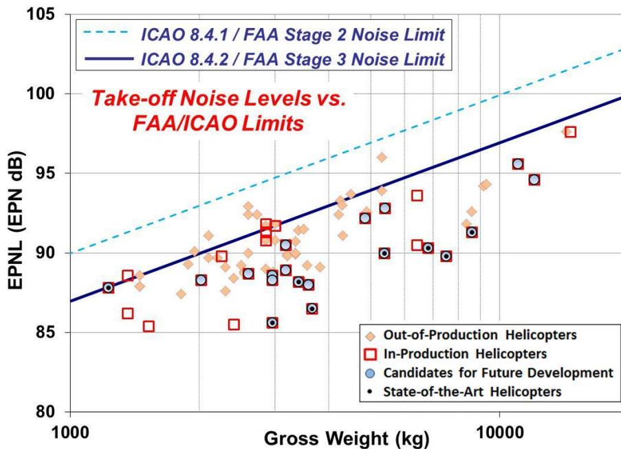
Figure A-1. Chapter 8 Take-off Certification Noise Levels vs. 8.4.1 and 8.4.2 Noise Limits
