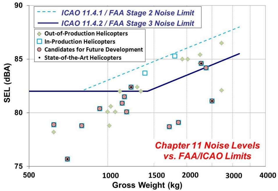
Figure A-4. Chapter 11 Certification Noise Levels vs. 11.4.1 and 11.4.2 Noise Limits
