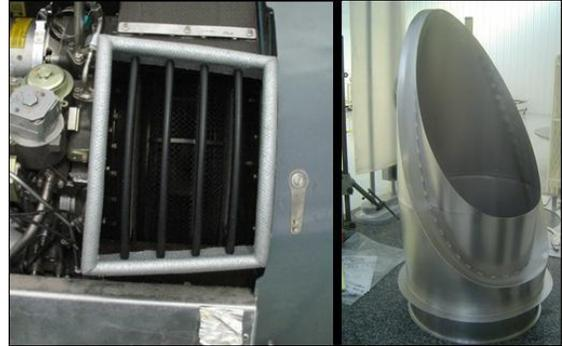
*Figures:* Acoustically treated additional lateral air inlet to the compressor chamber (left) and treated ejector (right)
