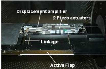
Wind Tunnel Test Model
