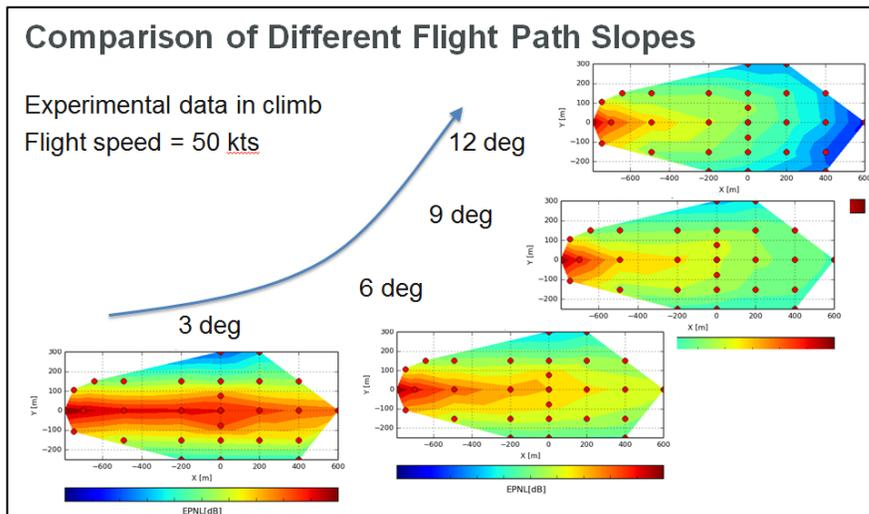
Figure: Comparison of Helicopter acoustic footprint at different climb slopes as measured in CleanSky
