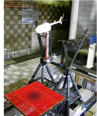
*Figure:* HELINOVI-Model in DNW-LLF wind tunnel
