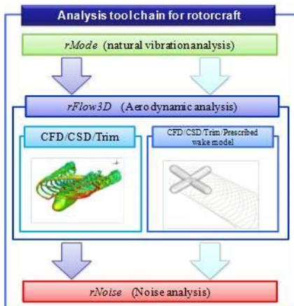
JAXA developed a CFD-based comprehensive analysis tool set (rFlow3D, rMode, and rNoise) to evaluate the aeroelastic behaviors of the rotor blade and to predict the rotor noise at an observation position, which has been used to evaluate the noise reduction capabilities of various active devices, including the HHC, active tab, active flap, and active twist.
