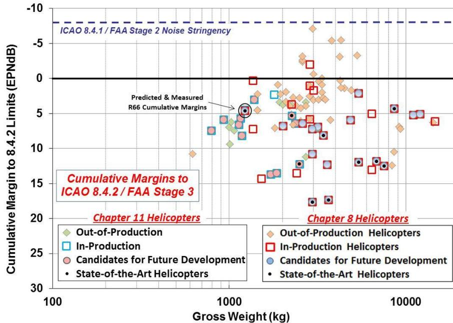
**Figure 3. Overlay of Predicted Chapter 11 Cumulative Margins with Chapter 8 Cumulative Margins**
