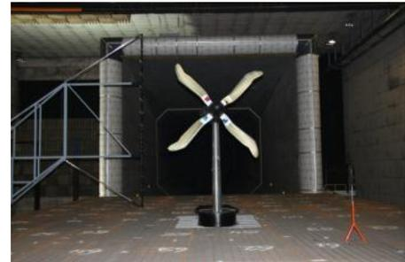
*Figure:* ADYN rotor in DNW-LLF wind tunnel
