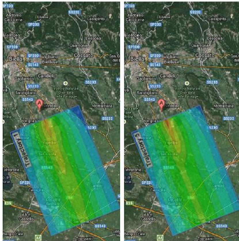
**Figure 9. Helicopter acoustic footprint for baseline (left) and steep (right) approach procedures located over the Biella airport (Italy), showing noise footprint reduction (green areas).**
