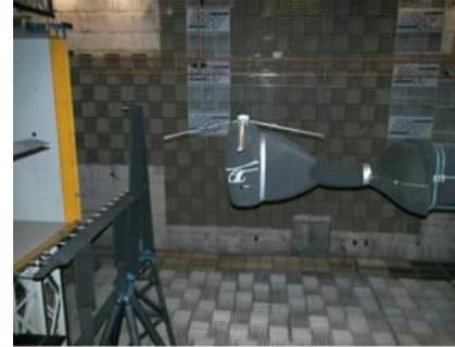
Model Rotor Testing at DNW
