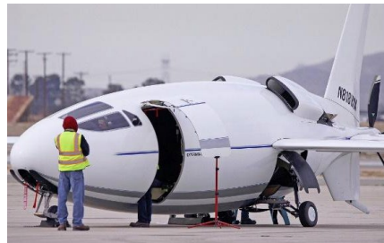
FIGURE 6: Otto Aviation Celera 500L laminar fuselage aircraft
