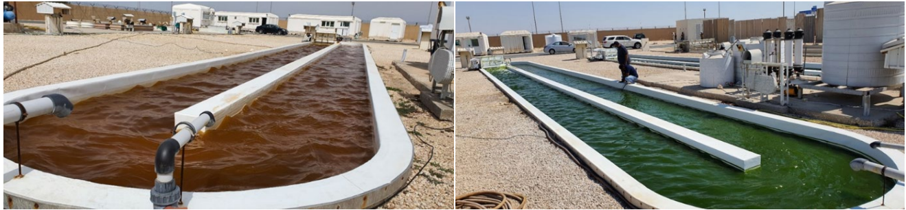
FIGURE 1: Lipid rich marine microalgae cultivated in 25,000 L outdoor open raceway ponds
